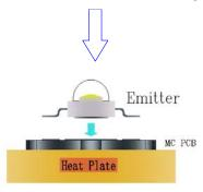
Put Emitter on MCPCB. Take the MCPCB out from Heat Plate within 10 seconds.
