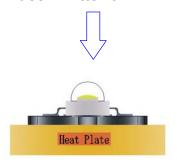
Put MCPCB on Heat Plate until Solder Paste melt. Put Emitter on MCPCB. Take the MCPCB out The Solder Paste sould be melted within 10 seconds. from Heat Plate within 10 seconds. Take out MCPCB out from Heat Plate within 10 seconds.
