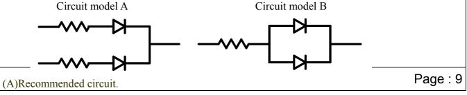
(B)The difference of brightness between LED's could be found due to the Vf-If characteristics of LED.
